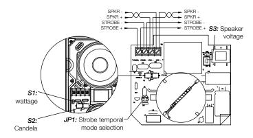
Genesis speaker-strobes may also be configured for temporal flash. This power-saving feature is intended for private mode signaling only. To set the device for temporal flash, snip the jumper at *JP1*.
