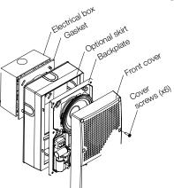
WG4 signals are rated for outdoor use and are suitable for indoor or outdoor applications on walls or ceilings. For surface-mounting in outdoor or wet applications, appliances must be mounted to a 449 or 74347U electrical box. In dry conditions, they are compatible with standard 4-inch by 1½-inch deep electrical boxes. When using the optional
